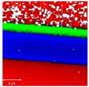
2D image of a cross section of a multilayered film, revealing the different layers of the polymer sample; polyethylene (PE) (red), titanium oxide ( $TiO_{e}$ ) (white), silicone, used as an adhesive (green), polyethylene terephthalate (blue).
