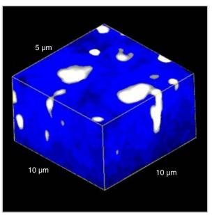
Volume image of a film revealing the 3D distribution and composition of the polypropylene (PP) (blue) and  $\text{TiO}_2$  (white).
