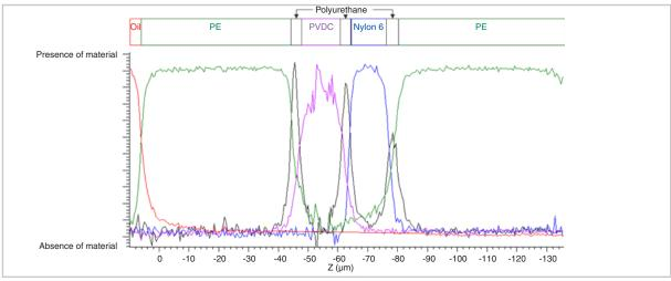
Depth profile of polymer laminate consisting of multiple layers: polyethylene (PE) (green), polyurethane (black), PVDC (pink), and Nylon 6 (blue), collected using an oil immersion objective. Z (in micrometres) refers to the depth penetrated in the sample (refractive index matched).
