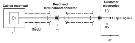
**IMPORTANT:** The shield should be connected to the machine earth (Field Ground).
