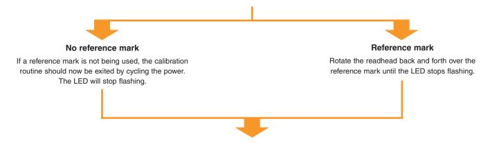
The system is now calibrated and ready for use. Calibration values, Automatic Gain Control (AGC) and Automatic Offset Control (AOC) status are stored in readhead non-volatile memory at power down.
