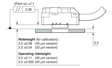
For detailed installation drawings, including tolerances, refer to www.renishaw.com/opticalencoders
