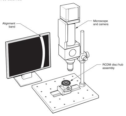
2 Rotate the disc/hub assembly and observe the maximum and minimum limits of movement of the alignment band as shown below.
