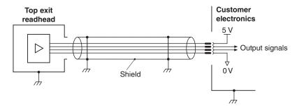
**IMPORTANT:** The shield should be connected to the machine earth (Field Ground).
