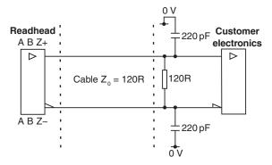
Standard RS422A line receiver circuitry Capacitors recommended for improved noise immunity
