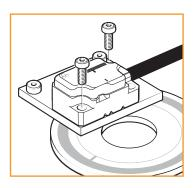
(7) Connect the readhead to the receiving electronics and power-up.
