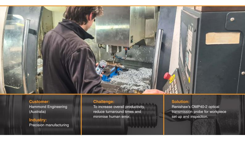
When Australia-based machine shop, Hammond Engineering, found that manually setting workpiece positions was time consuming and difficult to repeat, it looked to the potential of on-machine probing. Since using Renishaw's OMP40-2 optical transmission probe, the company has experienced faster set-up times and higher levels of productivity.
