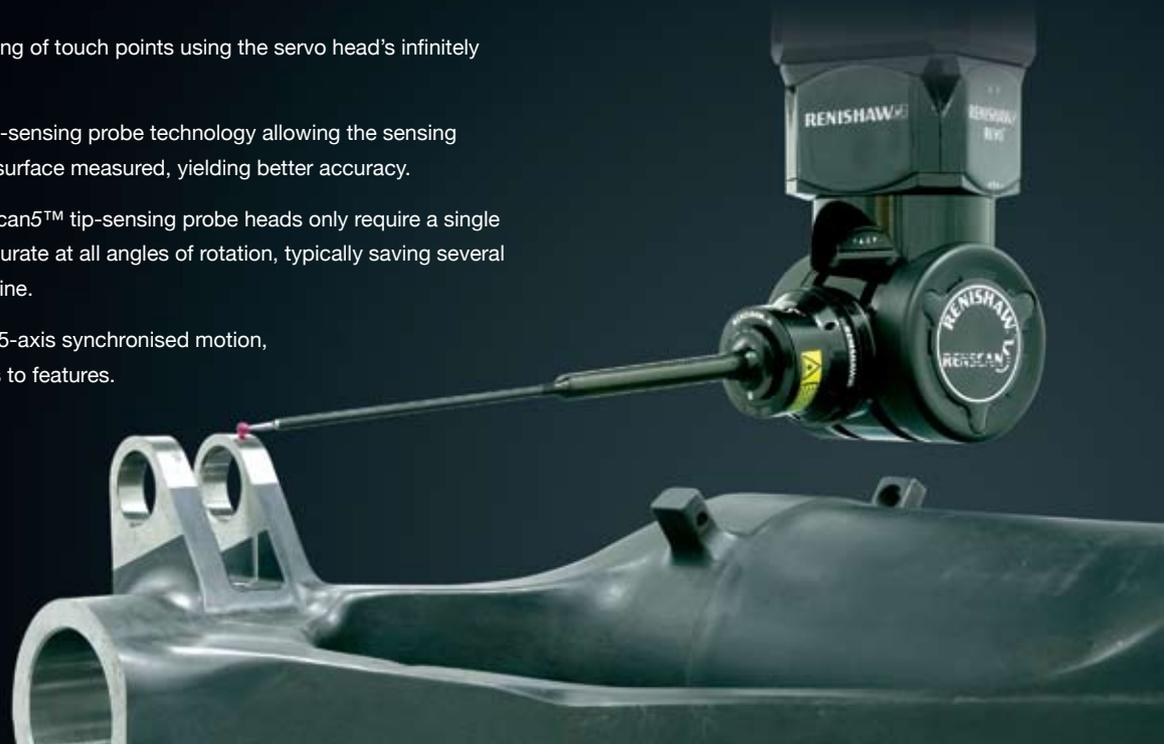
REVO™ 5-axis high speed, high accuracy measurement offers a wide range of benefits resulting in significant throughput improvements.
