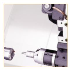
"The Renishaw probe allows our customer to machine and finish to size, cutting out the previous manual finishing operation"
