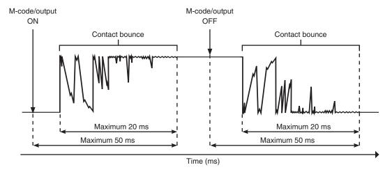
Any increase in these values will impact negatively on cycle times and may prevent the system working reliably.
